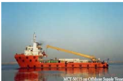
MCT-50115 on Offshore Supply Vessel 50T telescopic crane, 115 feet long, on Vicky II
