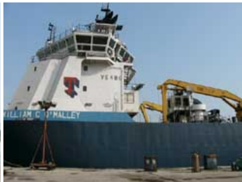
Alaska Marine Crane ® 25T knuckle boom crane, 52 feet long, on offshore supply vessel
