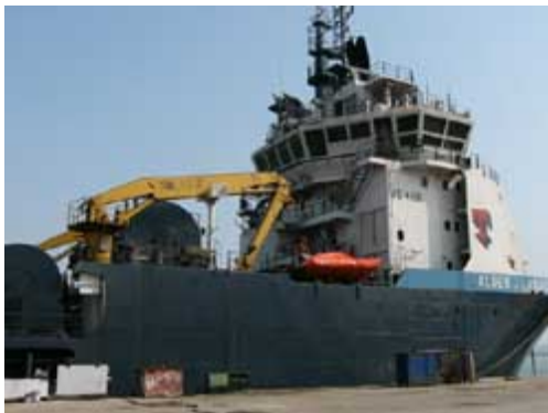
Alaska Marine Crane ® 25T knuckle boom crane, 52 feet long, on offshore supply vessel
